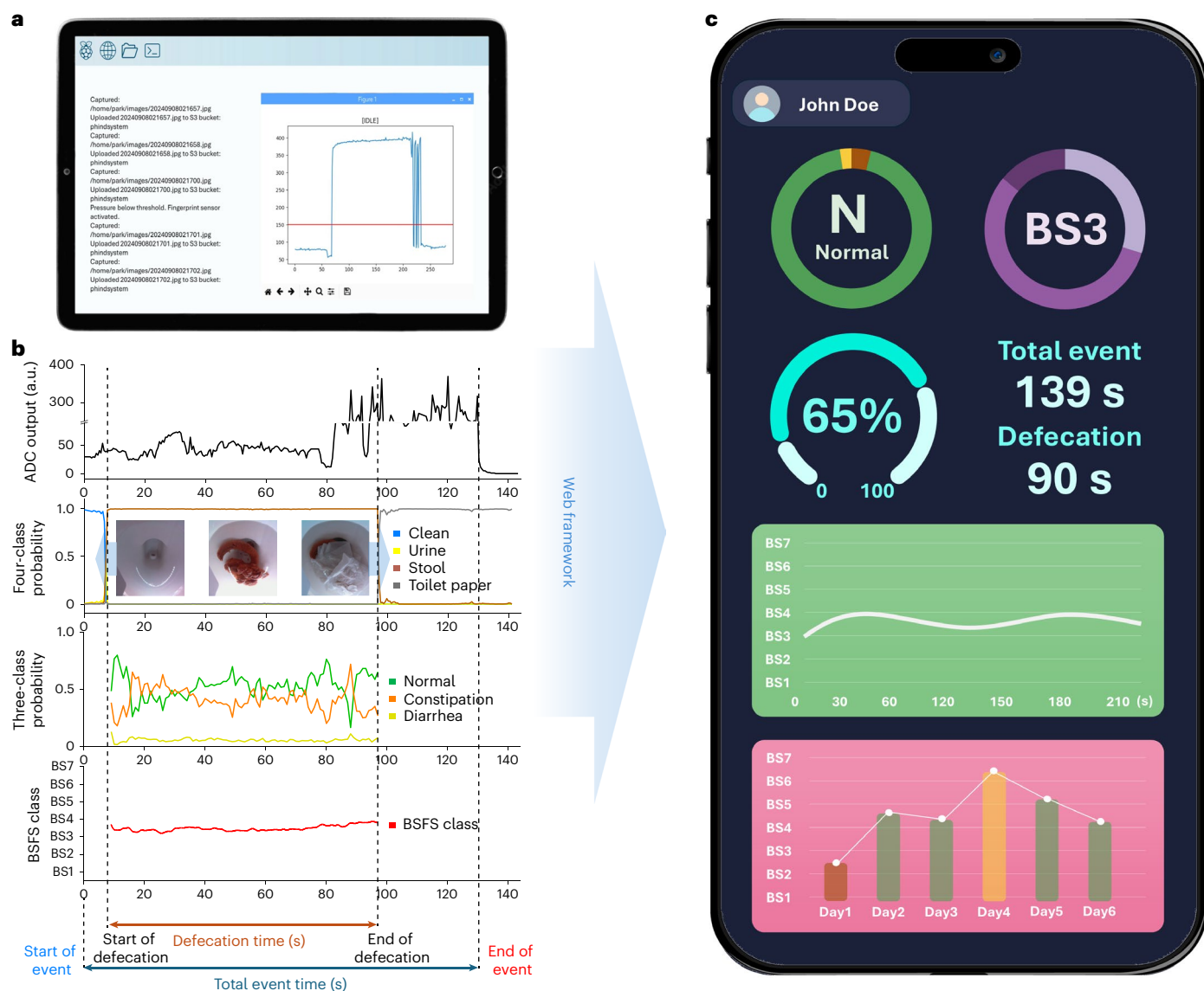
Fig. 10 | PHIND system UI. a , The screen shows a sample screen of the pressure sensor values and real-time data acquisition from the PHIND system. b , The acquired data analyzed within the cloud system. From top to bottom, the figures represent the pressure sensor graph to identify the start and end time of event,
